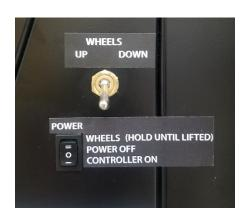
To power the system on, push the rocker switch down so that it is in the Controller On position.
