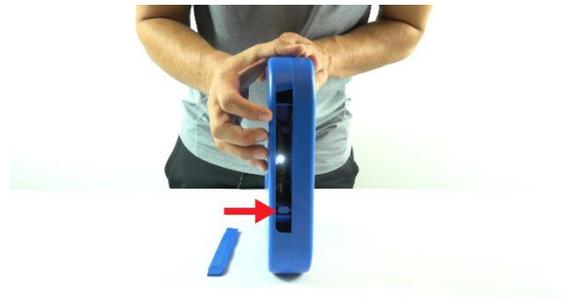
3. Hold the tab down and do not release it until you see the target display a T # and C #, then you can release the tab.
