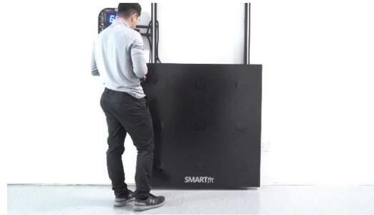
2. Apply direct constant pressure to the center of the panel. Hold this pressure while fully securing all 3 screws in each corner of the panel, then fully tighten the two remaining screws at the middle point of all 4 sides of the cover. This sequence of tightening the screws will eliminate the chance of air bubbles forming underneath the panel cover.
