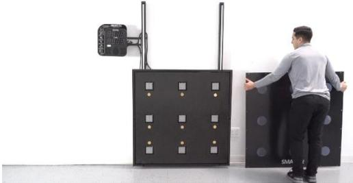
2. Turn on the CPU, then immediately and continuously tap the sensor connected to the target you wish to readdress.
