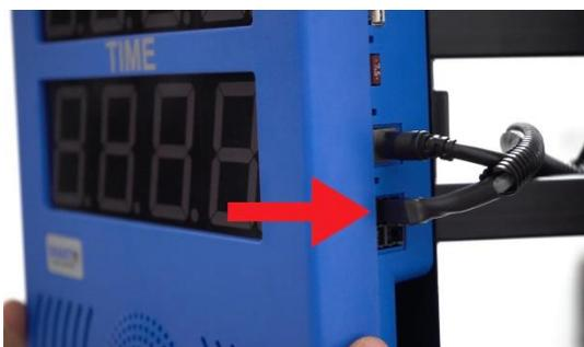
3. Flip the toggle switch to the on position. This switch will be located on the CPU when utilizing a Single or Mini installed on the wall. The same switch will be located on the side frame when utilizing a portable Mini and Single.
