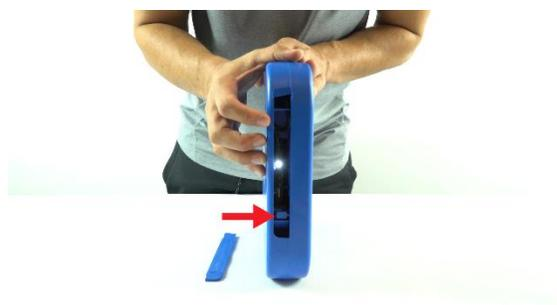
3. Hold the tab down and do not release it until you see the target display a T # and C #. You should release the tab when this displays on the target.
