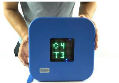
4. The target will display a T followed by a #. This number stands for the target number. Press the button once to change the target number. There are 31 target number options. Each strike Pod should have a different target number from each other.
